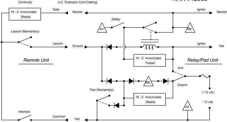
Test the cabling first with the safety switch open by toggling the Disarm/Arm switch. No sound is o.k. Repeat pressing test switch. Steady buzzer ONLY = o.k. battery in Disarm & o.k. igniter in Armed. Safety switch closed and fast pulsed and/or screeching sounds = Switch in disarm & good igniter. Slow pulsed sound = Switch in armed position. \*\*\*\* You should NEVER hear relay clicks during tests.
