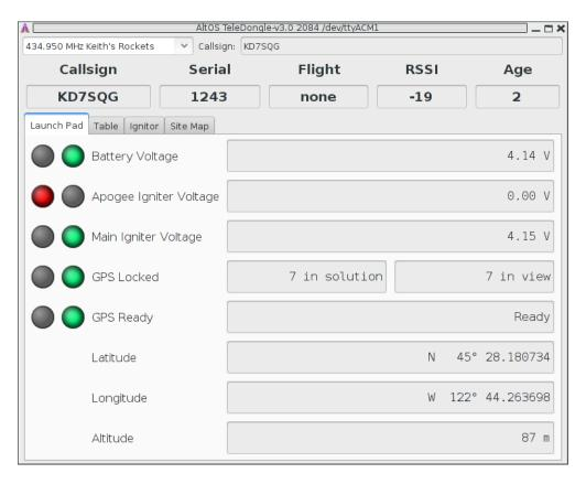
This brings up a dialog similar to the Monitor Flight UI, except it works with the altimeter in "idle" mode by sending query commands to discover the current state rather than listening for telemetry packets. Because this uses command mode, it needs to have the TeleDongle and flight computer callsigns match exactly. If you can receive telemetry, but cannot manage to run Monitor Idle, then it's very likely that your callsigns are different in some way.
