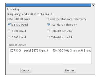
This listens for telemetry packets on all of the configured frequencies, displaying information about each device it receives a packet from. You can select which of the baud rates and telemetry formats should be tried; by default, it only listens at 38400 baud with the standard telemetry format used in v1.0 and later firmware.
