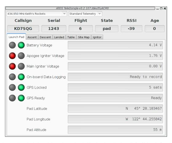
The 'Launch Pad' tab shows information used to decide when the rocket is ready for flight. The first elements include red/green indicators, if any of these is red, you'll want to evaluate whether the rocket is ready to launch:
