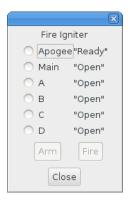
This activates the igniter circuits in the flight computer to help test recovery systems deployment. Because this command can operate over the Packet Command Link, you can prepare the rocket as for flight and then test the recovery system without needing to snake wires inside the air-frame.
