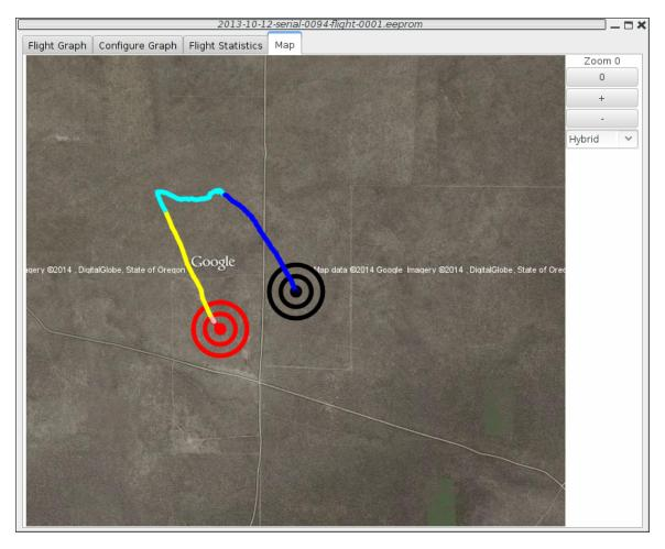
Shows a satellite image of the flight area overlaid with the path of the flight. The red concentric circles mark the launch pad, the black concentric circles mark the landing location.
