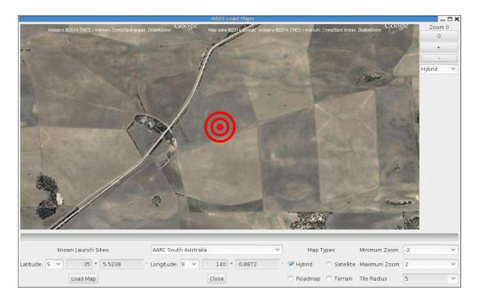
Before heading out to a new launch site, you can use this to load satellite images in case you don't have internet connectivity at the site. This loads a fairly large area around the launch site, which should cover any flight you're likely to make.
