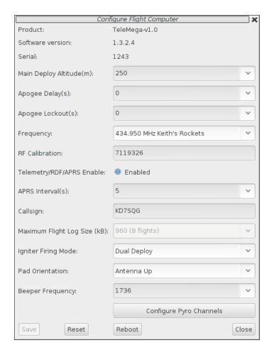
Select this button and then select either an altimeter or TeleDongle Device from the list provided. Selecting a TeleDongle device will use the radio link to configure a remote altimeter.
