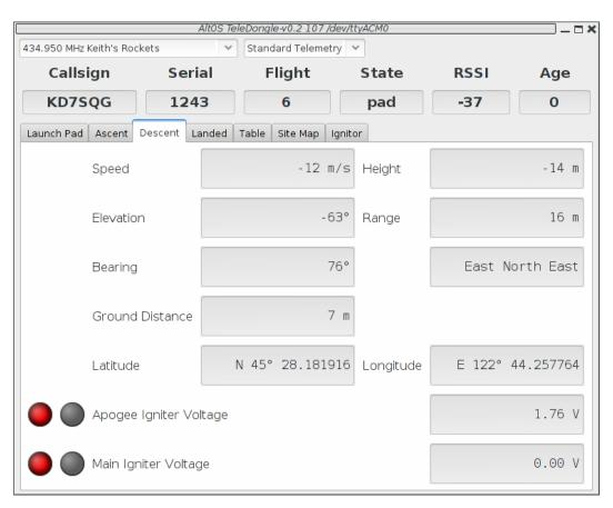
Once the rocket has reached apogee and (we hope) activated the apogee charge, attention switches to tracking the rocket on the way back to the ground, and for dual-deploy flights, waiting for the main charge to fire.
