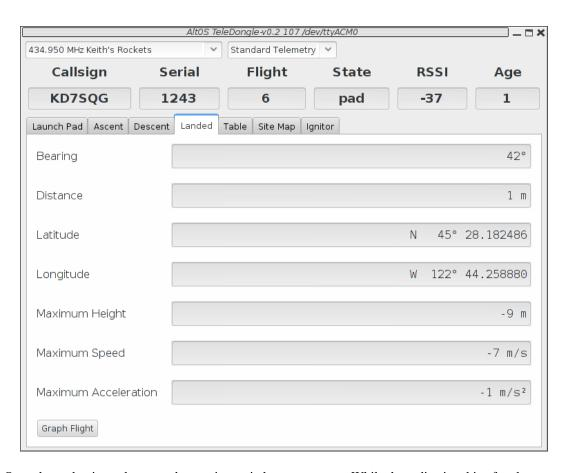
Once the rocket is on the ground, attention switches to recovery. While the radio signal is often lost once the rocket is on the ground, the last reported GPS position is generally within a short distance of the actual landing location.
