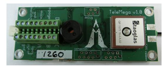
TeleMega is a 1¼ inch by 3¼ inch circuit board. It was designed to easily fit in a 38mm coupler. Like TeleMetrum, TeleMega has an accelerometer and so it must be mounted so that the board is aligned with the flight axis. It can be mounted either antenna up or down.
