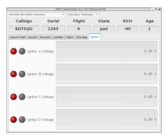
TeleMega includes four additional programmable pyro channels. The Ignitor tab shows whether each of them has continuity. If an ignitor has a low resistance, then the voltage measured here will be close to the pyro battery voltage. A value greater than 3.2V is required for a 'GO' status.
