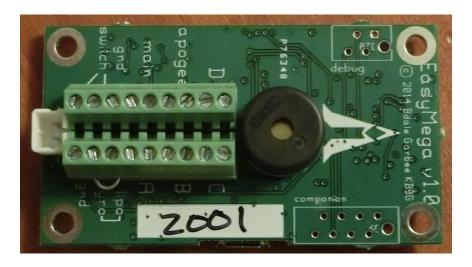
EasyMega is a 1¼ inch by 2¼ inch circuit board. It was designed to easily fit in a 38mm coupler. Like TeleMetrum, EasyMega has an accelerometer and so it must be mounted so that the board is aligned with the flight axis. It can be mounted either antenna up or down.
