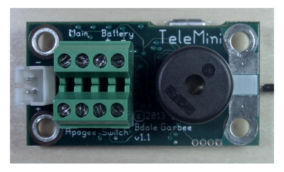
TeleMini v2.0 is 0.8 inches by 1½ inches. It adds more on-board data logging memory, a built-in USB connector and screw terminals for the battery and power switch. The larger board fits in a 24mm coupler. There's also a battery connector for a LiPo battery if you want to use one of those.
