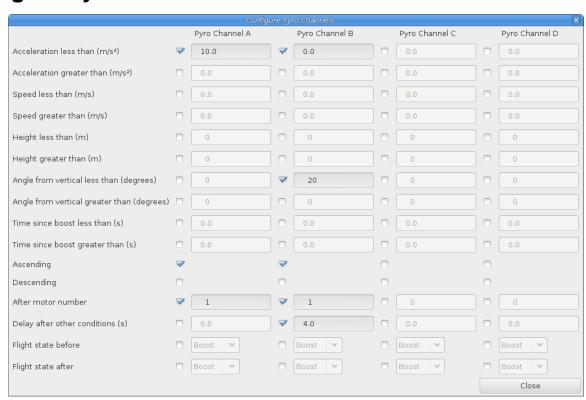
This opens a separate window to configure the additional pyro channels available on TeleMega. One column is presented for each channel. Each row represents a single parameter, if enabled the parameter must meet the specified test for the pyro channel to be fired. See the Pyro Channels section in the System Operation chapter above for a description of these parameters.
