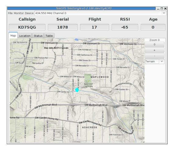
The map's default scale is approximately 3m (10ft) per pixel. The map can be dragged using the left mouse button. The map will attempt to keep the rocket roughly centered while data is being received.
