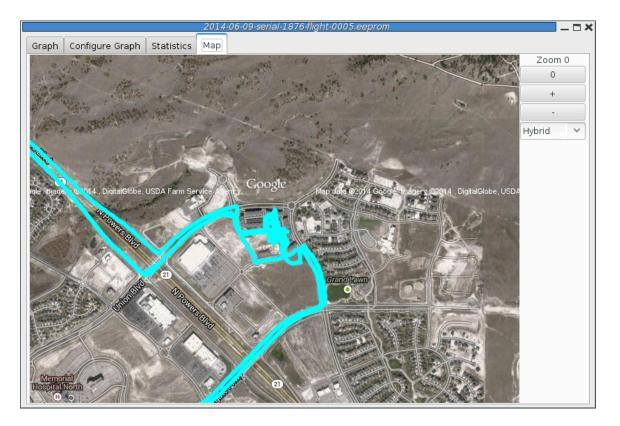
Shows a map of the area overlaid with the GPS track. As with the telemetry monitoring window, you can select the style of map and zoom level using buttons along the side; you can scroll the map by dragging within the map pressing the left button and you can draw a line to measure distances using either the left button with the shift key, or any other button.
