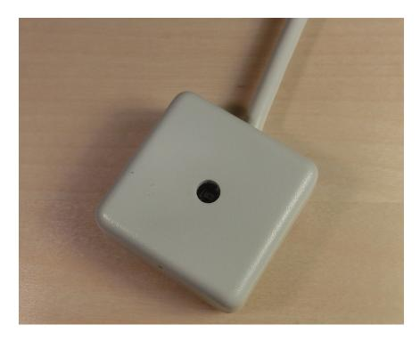
MicroPeak stores barometric pressure information for the first 48 seconds of the flight in on-board non-volatile memory. The contents of this memory can be downloaded to a computer using the MicroPeak USB adapter.
