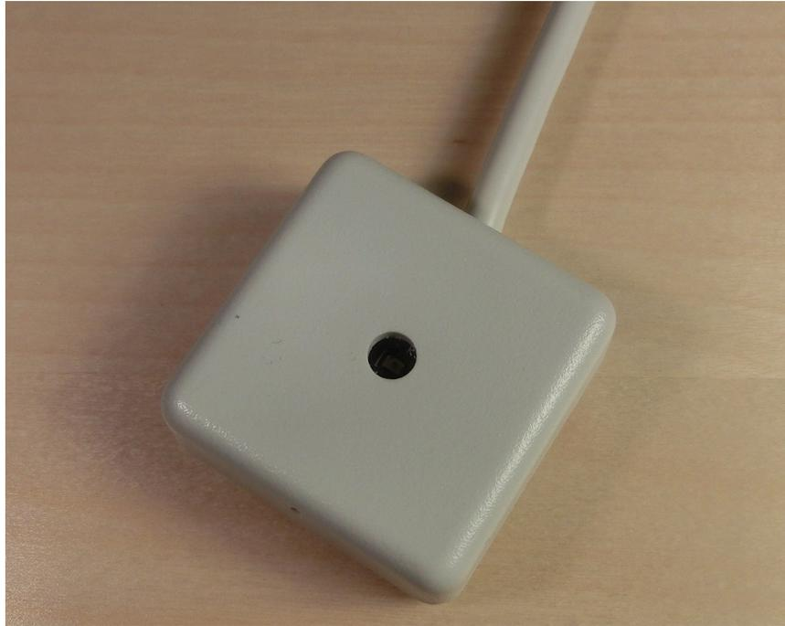
MicroPeak stores barometric pressure information for the first 48 seconds of the flight in on-board non-volatile memory. The contents of this memory can be downloaded to a computer using the MicroPeak USB adapter.
