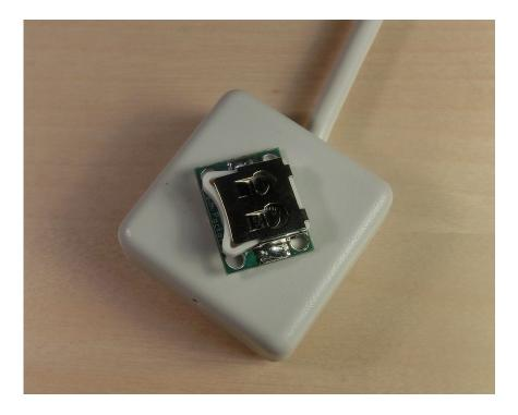
• After the maximum flight height is reported, MicroPeak will pause for a few seconds, blink the LED four times rapidly and then send the data in one long blur on the LED. The MicroPeak application should receive the data. When it does, it will present the data in a graph and offer to save the data to a file. If not, you can power cycle the MicroPeak board and try again.
