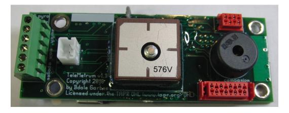
TeleMetrum is a 1 inch by 2¾ inch circuit board. It was designed to fit inside coupler for 29mm air-frame tubing, but using it in a tube that small in diameter may require some creativity in mounting and wiring to succeed! The presence of an accelerometer means TeleMetrum should be aligned along the flight axis of
