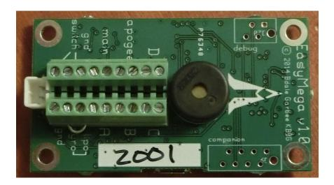
EasyMega is a 1¼ inch by 2¼ inch circuit board. It was designed to easily fit in a 38mm coupler. Like TeleMetrum, EasyMega has an accelerometer and so it must be mounted so that the board is aligned with the flight axis. It can be mounted either antenna up or down.
