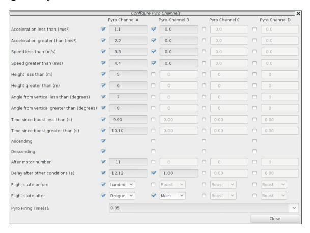
This opens a separate window to configure the additional pyro channels available on TeleMega and EasyMega. One column is presented for each channel. Each row represents a single parameter, if enabled the parameter must meet the specified test for the pyro channel to be fired. See the Pyro Channels section in the System Operation chapter above for a description of these parameters.
