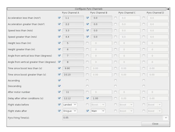
This opens a separate window to configure the additional pyro channels available on TeleMega. One column is presented for each channel. Each row represents a single parameter, if enabled the parameter must meet the specified test for the pyro channel to be fired. See the Pyro Channels section in the System Operation chapter above for a description of these parameters.
