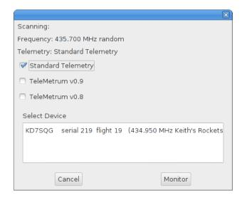
This listens for telemetry packets on all of the configured frequencies, displaying information about each device it receives a packet from. You can select which of the three telemetry formats should be tried; by default, it only listens for the standard telemetry packets used in v1.0 and later firmware.
