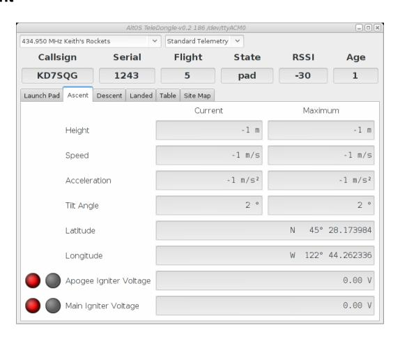
This tab is shown during Boost, Fast and Coast phases. The information displayed here helps monitor the rocket as it heads towards apogee.
