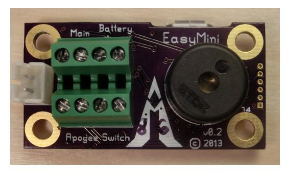
EasyMini is built on a 0.8 inch by 1½ inch circuit board. It's designed to fit in a 24mm coupler tube. The connectors and screw terminals match TeleMini v2.0, so you can easily swap between EasyMini and TeleMini.
