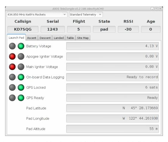
The 'Launch Pad' tab shows information used to decide when the rocket is ready for flight. The first elements include red/green indicators, if any of these is red, you'll want to evaluate whether the rocket is ready to launch:
