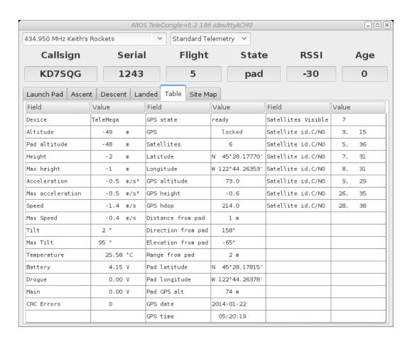
The table view shows all of the data available from the flight computer. Probably the most useful data on this tab is the detailed GPS information, which includes horizontal dilution of precision information, and information about the signal being received from the satellites.
