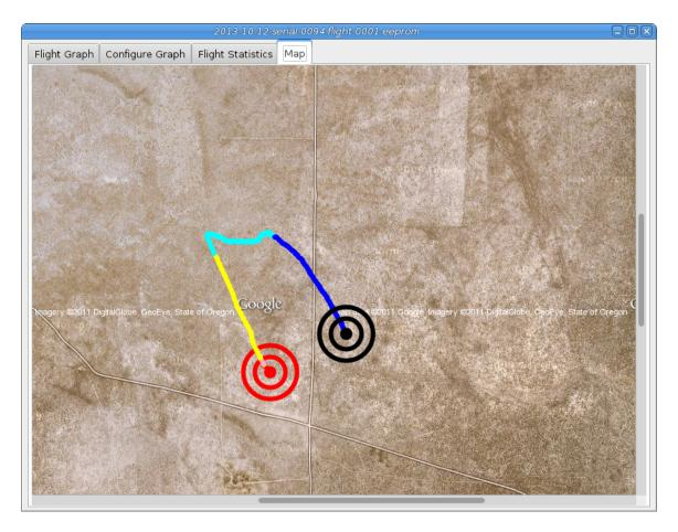
Shows a satellite image of the flight area overlaid with the path of the flight. The red concentric circles mark the launch pad, the black concentric circles mark the landing location.
