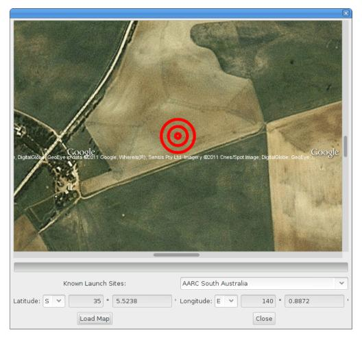
Before heading out to a new launch site, you can use this to load satellite images in case you don't have internet connectivity at the site. This loads a fairly large area around the launch site, which should cover any flight you're likely to make.
