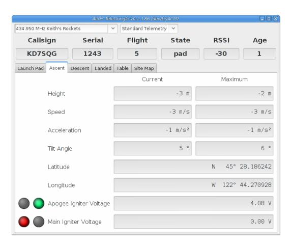
This tab is shown during Boost, Fast and Coast phases. The information displayed here helps monitor the rocket as it heads towards apogee.
