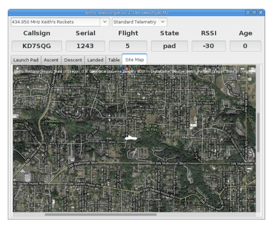
When the TeleMetrum has a GPS fix, the Site Map tab will map the rocket's position to make it easier for you to locate the rocket, both while it is in the air, and when it has landed. The rocket's state is indicated by color: white for pad, red for boost, pink for fast, yellow for coast, light blue for drogue, dark blue for main, and black for landed.
