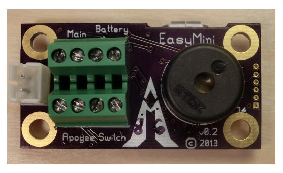
EasyMini is built on a 0.8 inch by  $1\frac{1}{2}$  inch circuit board. It's designed to fit in a 24mm coupler tube. The connectors and screw terminals match TeleMini v2.0, so you can easily swap between EasyMini and TeleMini.
