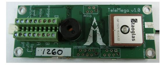
TeleMega is a 1¼ inch by 3¼ inch circuit board. It was designed to easily fit in a 38mm coupler. Like TeleMetrum, TeleMega has an accelerometer and so it must be mounted so that the board is aligned with the flight axis. It can be mounted either antenna up or down.
