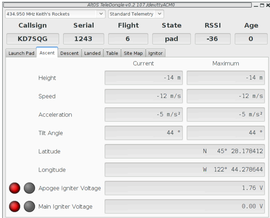
Figure 11.4. Monitor Flight Ascent View
