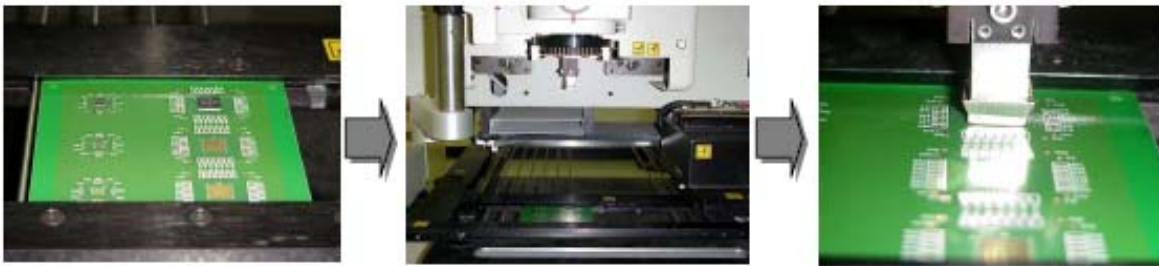
Figure 13. QFN Package Removal Process
