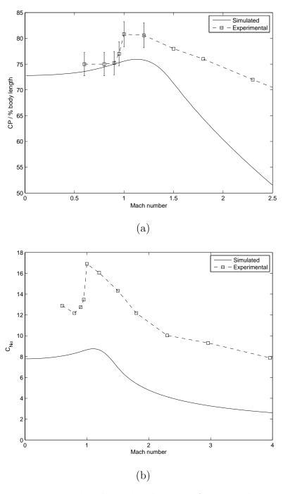
Figure 6.7: Experimental and simulated center of pressure location (a) and normal force coefficient derivative (b) as a function of Mach number.
