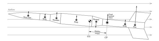
Figure 2.4: Normal forces produced by the rocket components.
