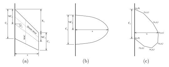
Figure 3.2: Fin geometry of (a) a trapezoidal fin, (b) an elliptical fin and (c) a free-form fin.
