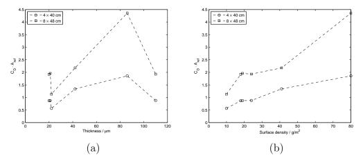
Figure C.3: The normalized drag coefficient of a streamer as a function of (a) the material thickness and (b) the material surface density.
