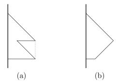
Figure 3.3: (a) A jagged fin edge, and (b) an equivalent fin if c(y) is chosen to include only the actual fin area.
