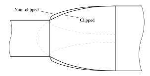
Figure A.2: A clipped and non-clipped elliptical transition.
