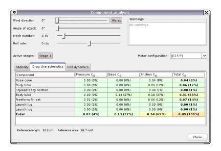
Figure 5.3: Dialog windows for editing the properties of a nose cone and for analyzing the influence of individual components on the stability, drag and roll characteristics of the rocket.
