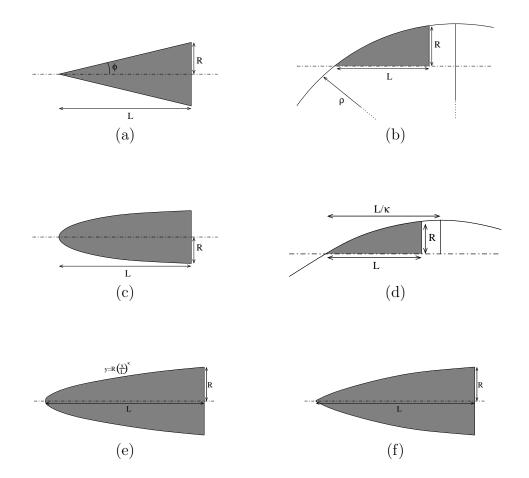
Figure A.1: Various nose cone geometries: (a) conical, (b) secant ogive, (c) elliptical, (d) parabolic, (e) 1/2 power (ellipsoid) and (f) Haack series (Von Kárman).
