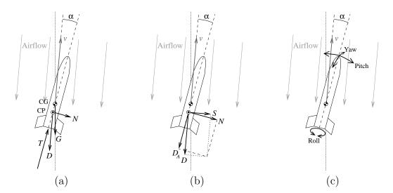
Figure 3.1: (a) Forces acting on a rocket in free flight: gravity G, motor thrust T, drag D and normal force N. (b) Perpendicular component pairs of the total aerodynamical force: normal force N and axial drag  $D_A$ ; side force S and drag D. (c) The pitch, yaw and roll directions of a model rocket.
