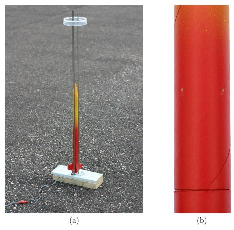
Figure 6.1: The test rocket awaiting launch on the tower launcher (a) and a close-up of its ventilation holes (b).
