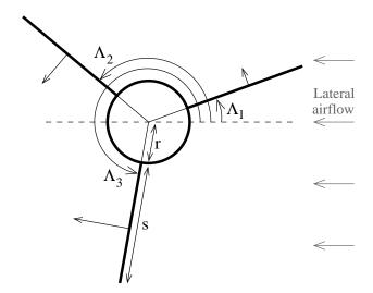
Figure 3.6: The geometry of an uncanted three-fin configuration (viewed from rear).
