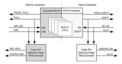
Figure 4-3: Functional Implementation of Built-in FIFO
