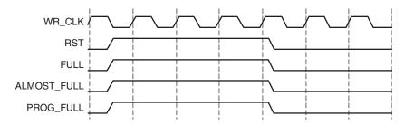
Figure 4-24: Block RAM, Distributed RAM, Shift RAM with Full Flags Reset Value of 1
