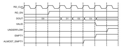
Figure 4-8: FWFT Read Operation for a FIFO with Independent Clocks
