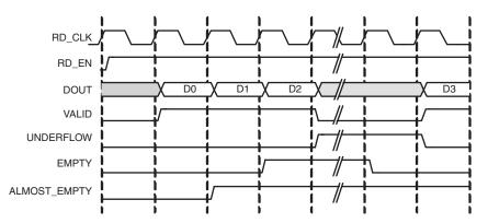
Figure 4-7: Standard Read Operation for a FIFO with Independent Clocks
