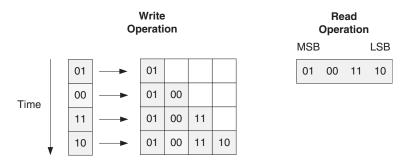
Figure 4-17: 1:4 Aspect Ratio: Data Ordering
