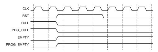
Figure 4-26: Built-in FIFO, Asynchronous Reset Behavior
