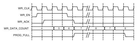
Figure 4-12: Programmable Full Single Threshold: Threshold Set to 7
