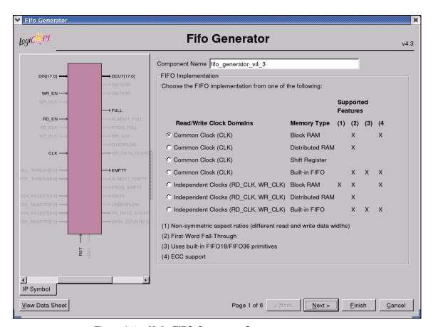
Figure 3-1: Main FIFO Generator Screen
