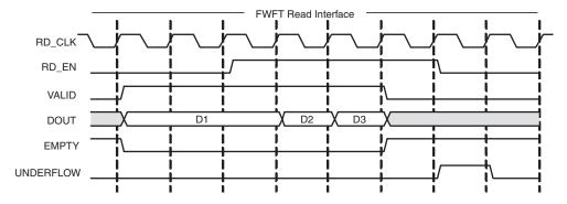
Figure 4-10: Handshaking Signals for a FIFO with Independent Clocks
