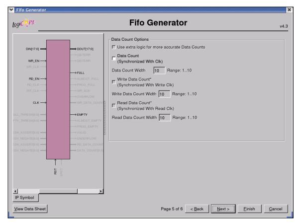
Figure 3-5: Data Count and Reset Screen
