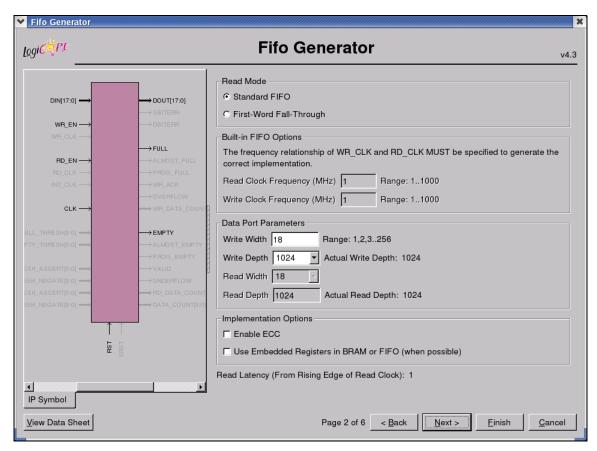
Figure 3-2: Performance Options and Data Port Parameters Screen
