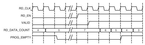
Figure 4-14: Programmable Empty with Single Threshold: Threshold Set to 4
