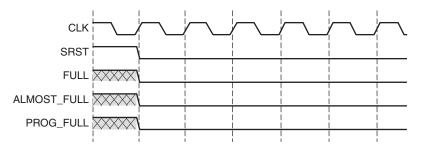
Figure 4-27: Synchronous Reset: FIFO with a Common Clock
