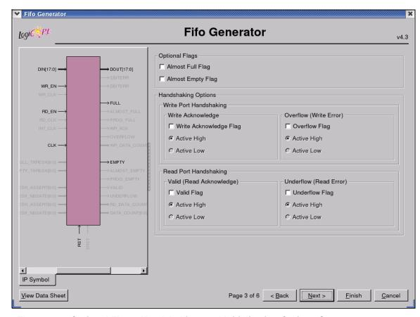
Figure 3-3: Optional Flags, Handshaking, and Initialization Options Screen
