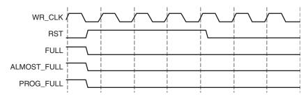
Figure 4-25: Block RAM, Distributed RAM, Shift RAM with Full Flags Reset Value of 0
