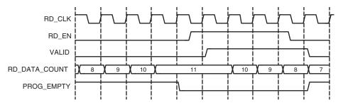
Figure 4-15: Programmable Empty with Assert and Negate Thresholds: Assert Set to 7 and Negate Set to 10
