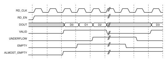
Figure 4-21: Standard Read Operation for a block RAM or built-in FIFO with Use Embedded Registers Enabled
