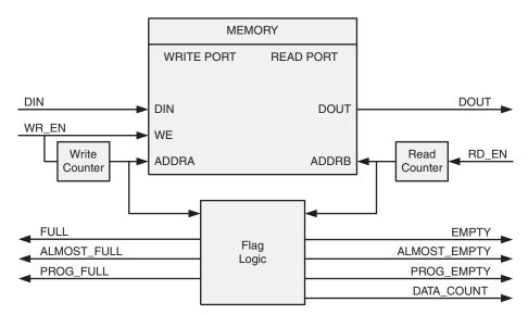
Figure 4-4: Functional Implementation of a Common Clock FIFO using Block RAM or Distributed RAM
