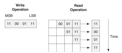
Figure 4-19: 4:1 Aspect Ratio: Data Ordering
