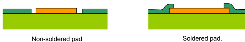
Figure 22: Solder mask openings for copper pads.
