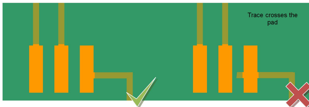
Figure 10: Starting position of the trace to the pad.
