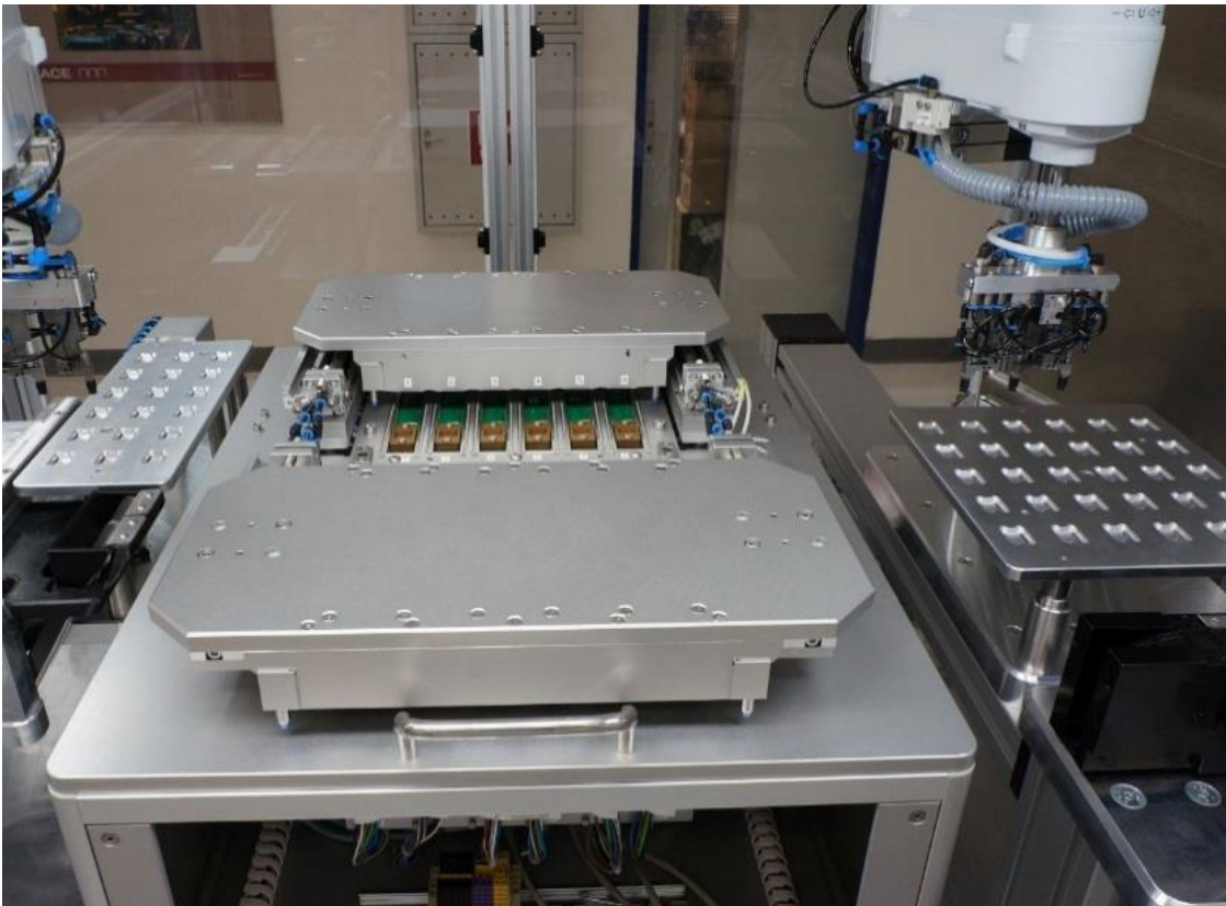
Figure 27: Automatic test equipment for module test
