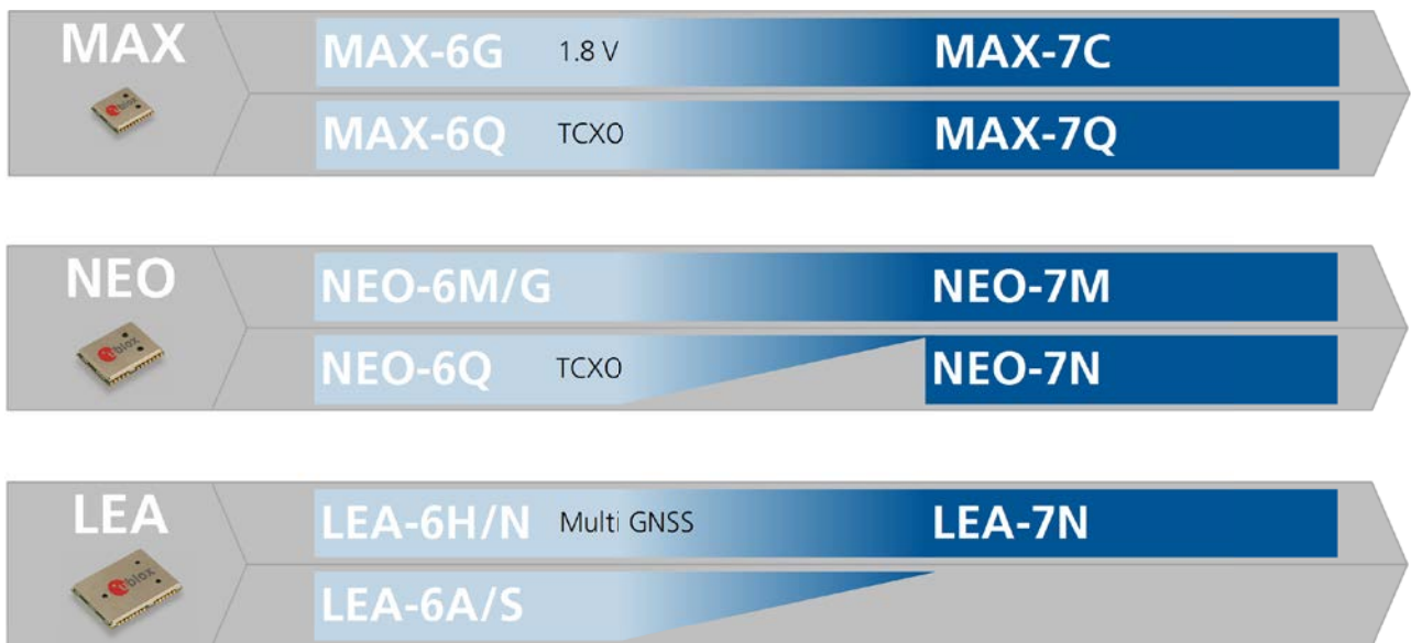
Figure 33: Migrating u-blox 6 designs to a u-blox 7 receiver module
