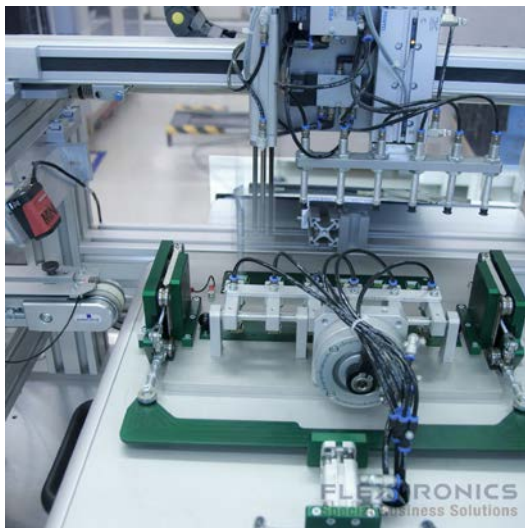
Figure 42: Automatic Test Equipment for Module Tests
