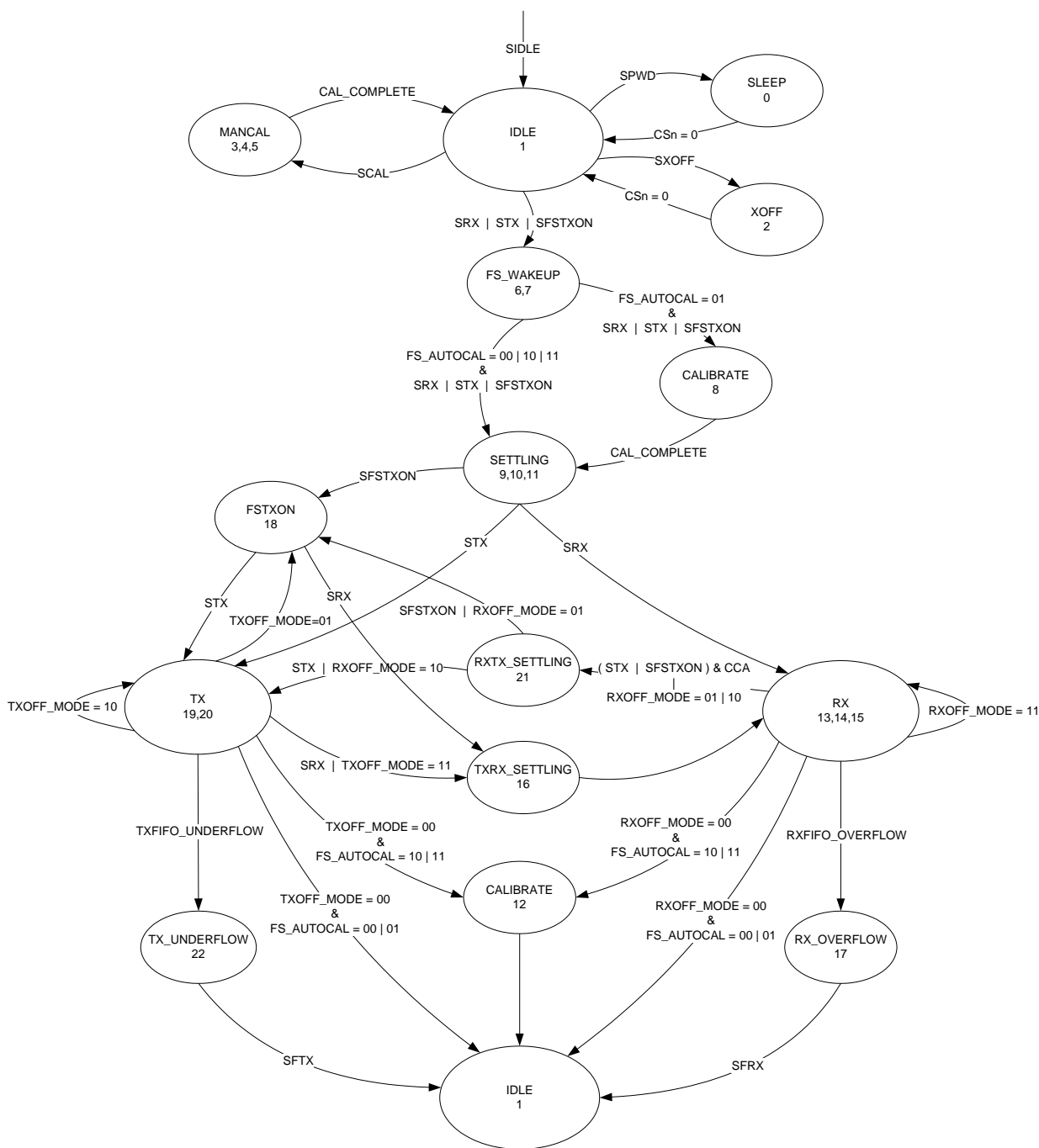
Figure 19: Complete Radio Control State Diagram
