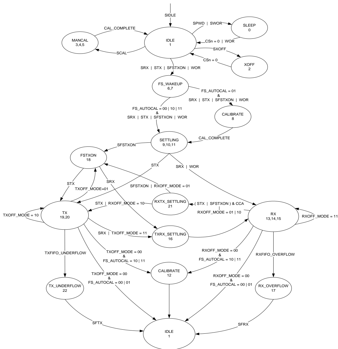
Figure 25: Complete Radio Control State Diagram
