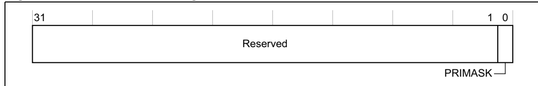
Figure 5. PRIMASK bit assignments
