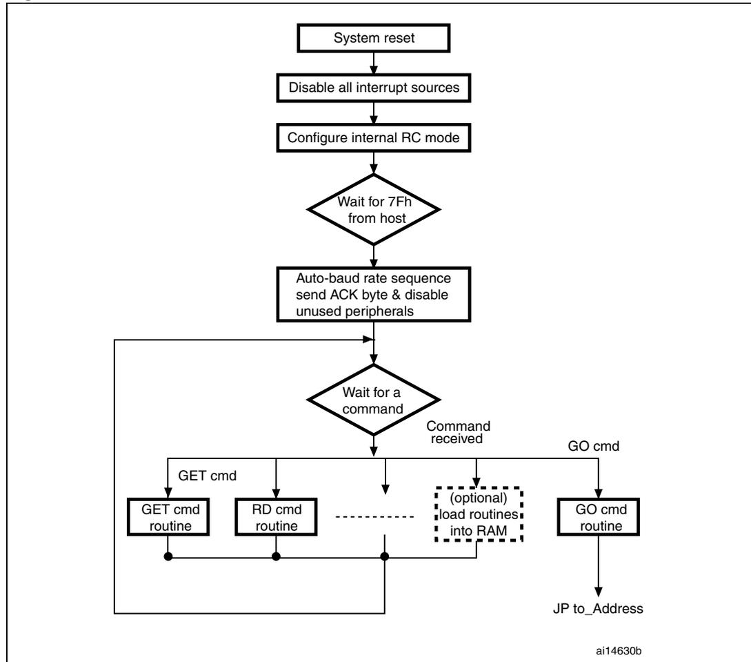
Once System memory boot mode is entered and the microcontroller has been configured as described above, the bootloader code begins to scan the USART1\_RX line pin, waiting to receive the 0x7F data frame: one start bit, 0x7F data bits, even parity bit and one stop bit.
