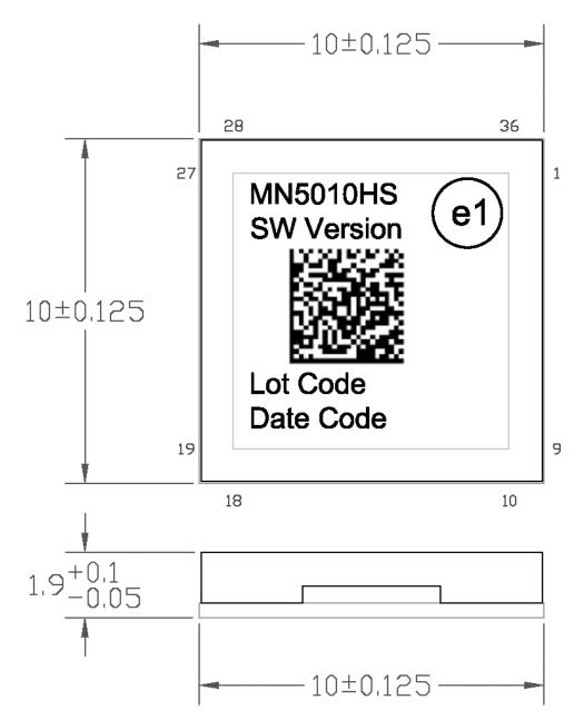
Figure 3 – Package Outline & Marking (in mm) : 36-pin LGA Note the JEDEC Pb-free symbol is also used as the pin 1 identifier for the MN5010HS.
