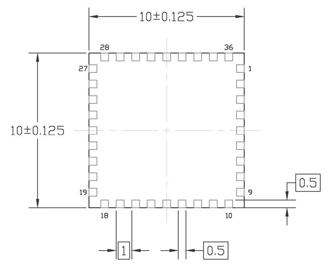
Figure 4 – Recommended PCB Footprint (in mm) – Top View
