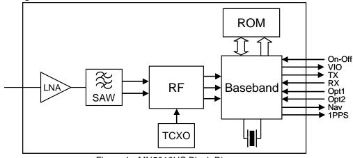
Figure 1 - MN5010HS Block Diagram
