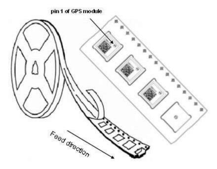
Figure 7 – Orientation in tape
