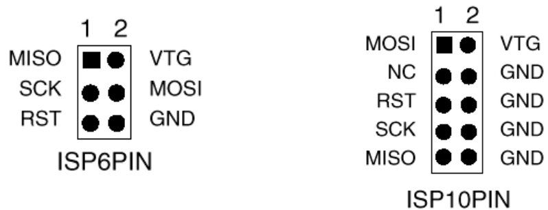
Figure 4-1. Standard ISP connectors on STK500, AVR ISP and STK200/STK300
